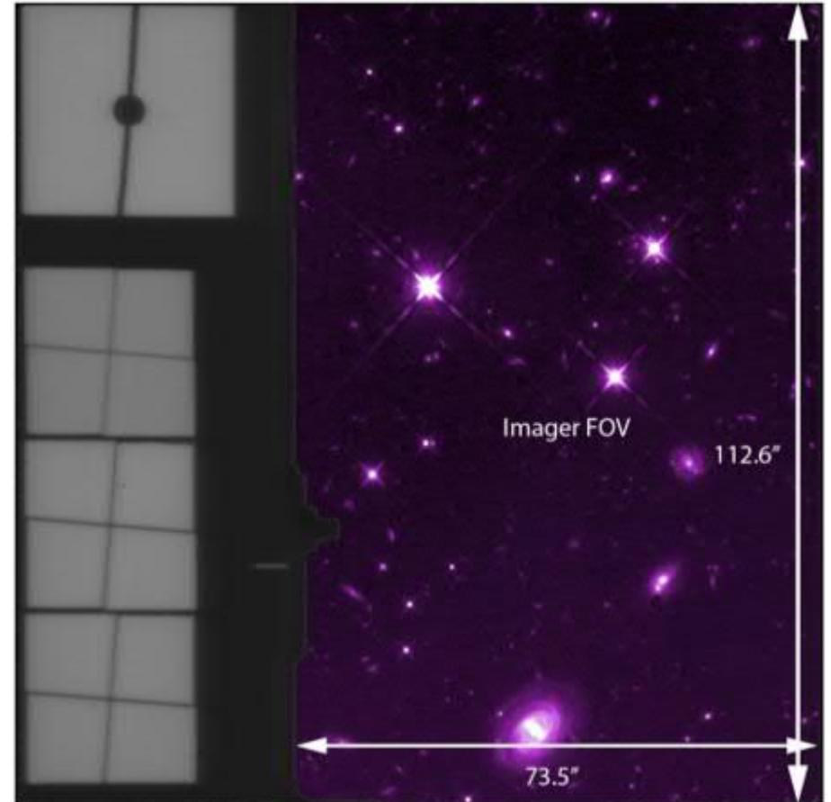
The imager has a plate scale of 0.11 arcseconds/pixel and a field of view of 74 by 113 arcseconds with filters ranging from 5.6 to 25.5  $\mu\text{m}$ . It has a 1024x1024 pixel array of arsenic doped silicon pixels.
