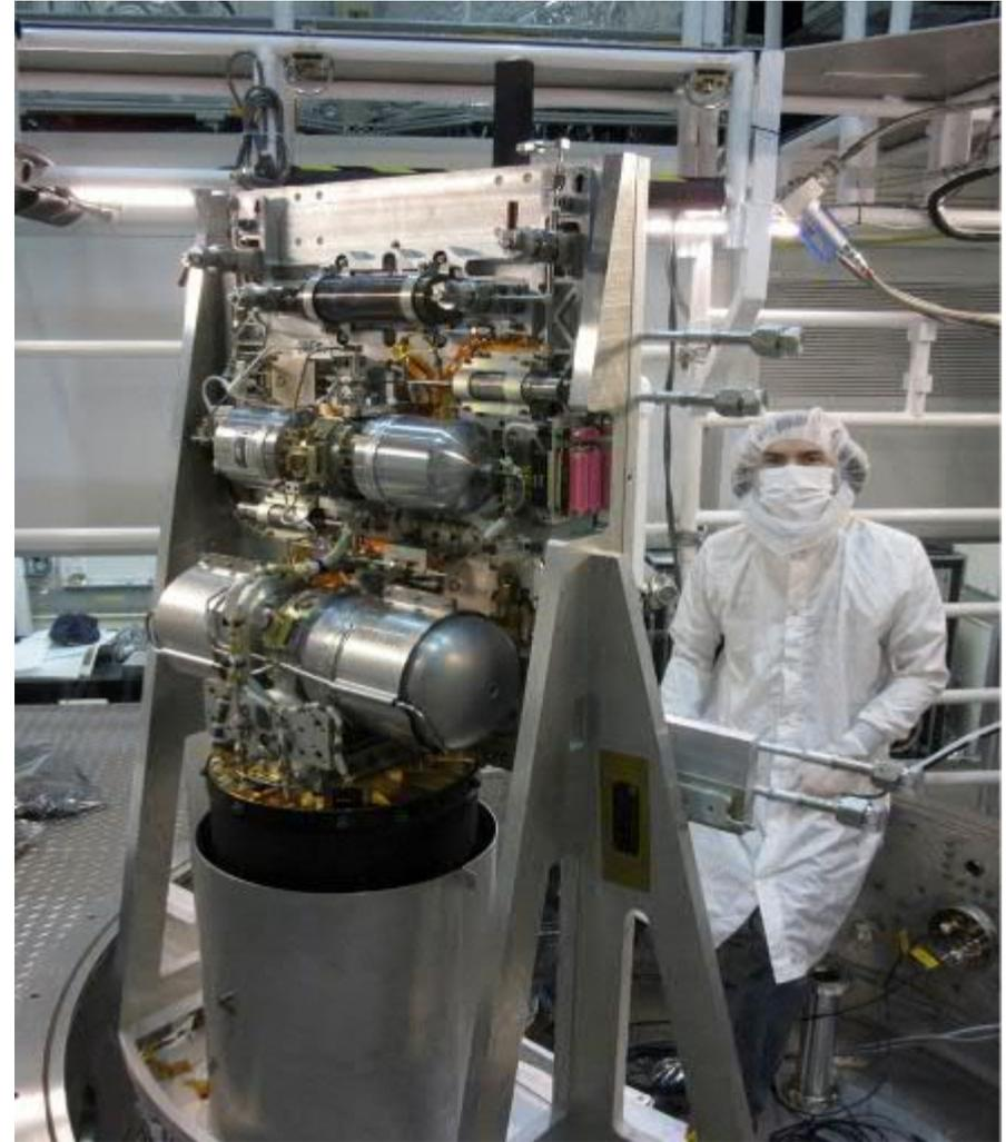
The MIRI instrument. MIRI's operates at temperatures of no more than 6.7 degrees above absolute zero.
