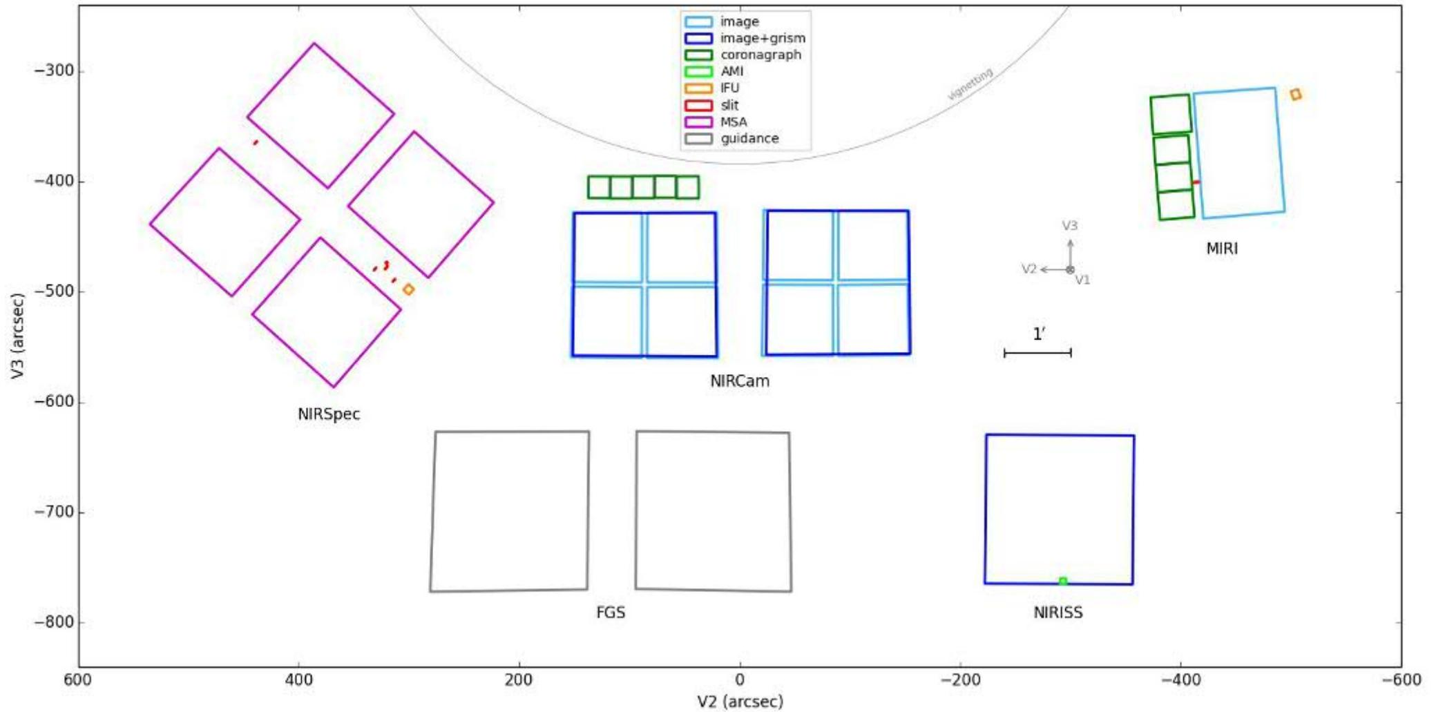
The ISIM instruments are located in an off-axis position, which yield excellent image quality over the 9.4 arcminute field
