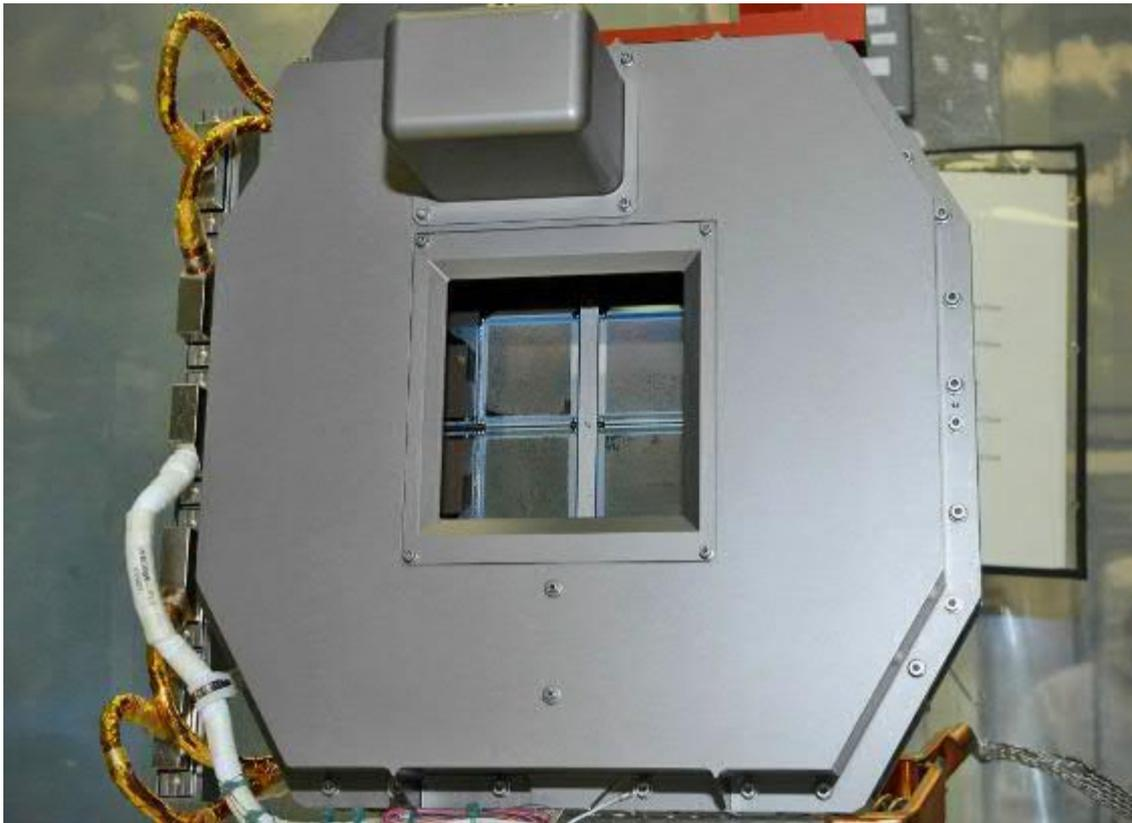
Multi-object spectroscopy obtains simultaneous spectroscopy of multiple science targets within a  $3.6 \times 3.4'$  field of view using the micro-shutter assembly (MSA)
