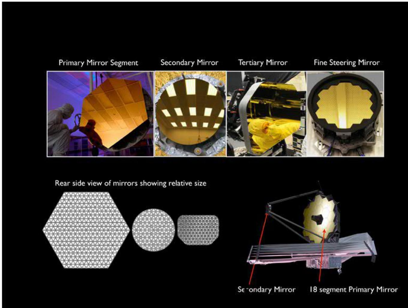
Fine steering mirror (FSM) with line-of-sight (LOS) stabilization  $< 7.3$  marcsec (or mas).
